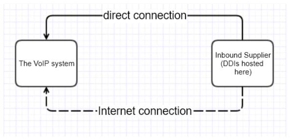
In the figure above inbound traffic would normally be delivered by the direct connection, but in the event of failure, calls would be delivered across the internet.
