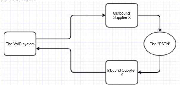
The figure above shows a typical call route for monitoring the quality of calls; the call is sent out on supplier X and is subsequently received from supplier Y. By use of a combination of routine calls the connection that is causing a quality failure can be established.
