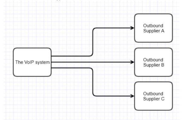
The figure above shows a possible routing plan where 3 different suppliers are available, which supplier is chosen for a call is likely to depend on cost and quality issues but if a supplier becomes unavailable, then other suppliers are available to handle the call.
